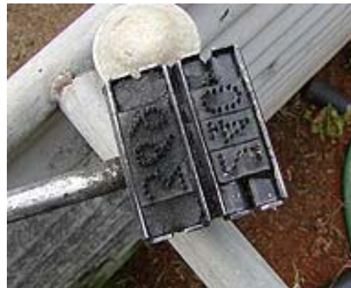
Figure 1. Swine brand in good condition – no bent or missing needles
